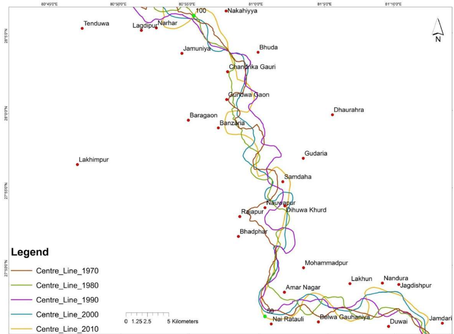
Figure 7.14a Shifting of center line of Sharda river from chainage 50-100 km
